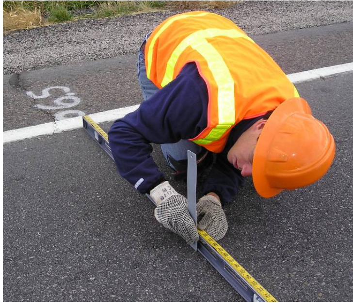
Figure 3.5 Measurement of Rut Depth
