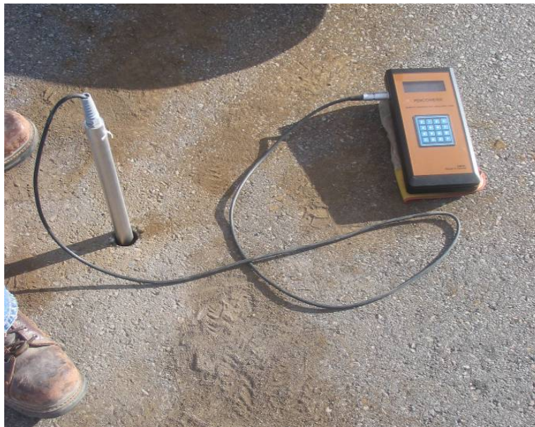
Figure 3.8 Measurement of Electrical Properties
