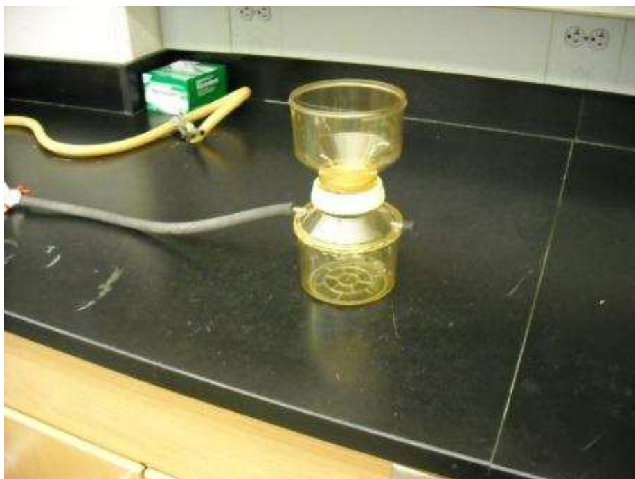
Figure 3.4: Apparatus Used in Vacuum Filtration of Prepared Solutions
