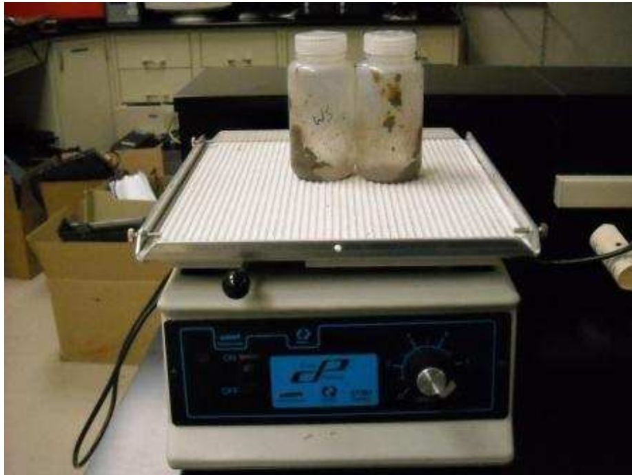
Figure 3.3: Shaker Table and Tubes Used in Fractionation
