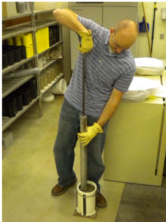
Figure 3.7: Preparation of sample for hydraulic conductivity testing.
