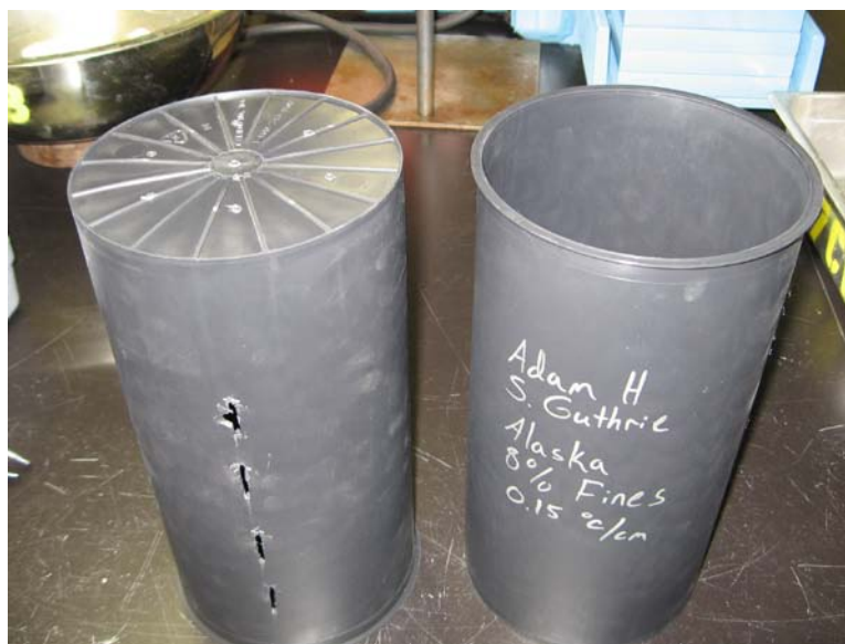
Figure 3.1: Sample molds for frost heave testing.
