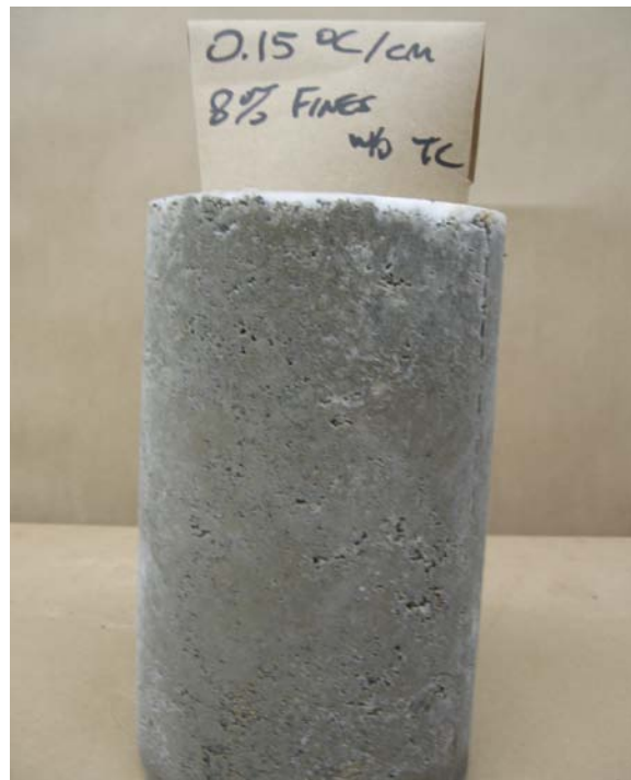
Figure A.13: Specimen with 8 percent fines tested without thermocouples at thermal gradient of 0.15^{\circ}\text{C}/\text{cm} .
