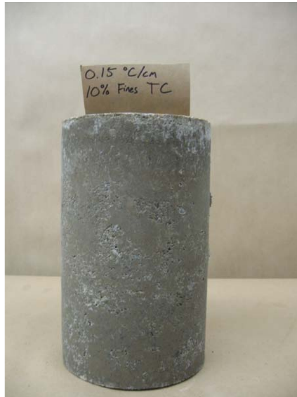
Figure A.16: Specimen with 10 percent fines tested with thermocouples at thermal gradient of 0.15^{\circ}\text{C}/\text{cm} .
