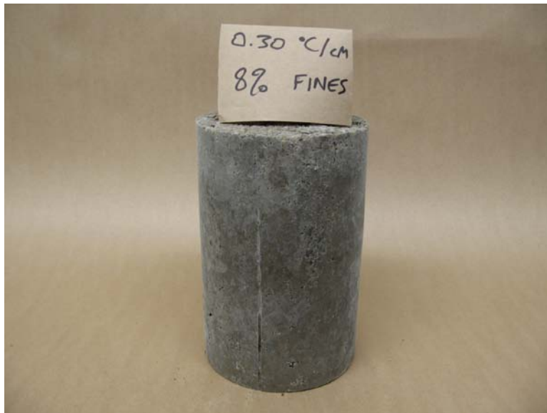
Figure A.19: Specimen with 8 percent fines tested without thermocouples at thermal gradient of 0.30^{\circ}\text{C}/\text{cm}
