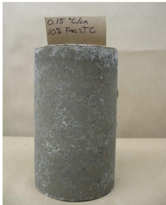
Figure A.15: Specimen with 10 percent fines tested without thermocouples at thermal gradient of 0.15^{\circ}\text{C}/\text{cm} .
