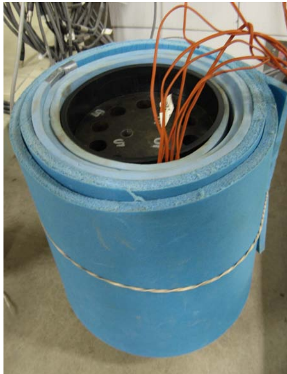
Figure 3.3: Sample with insulation and overburden weight.
