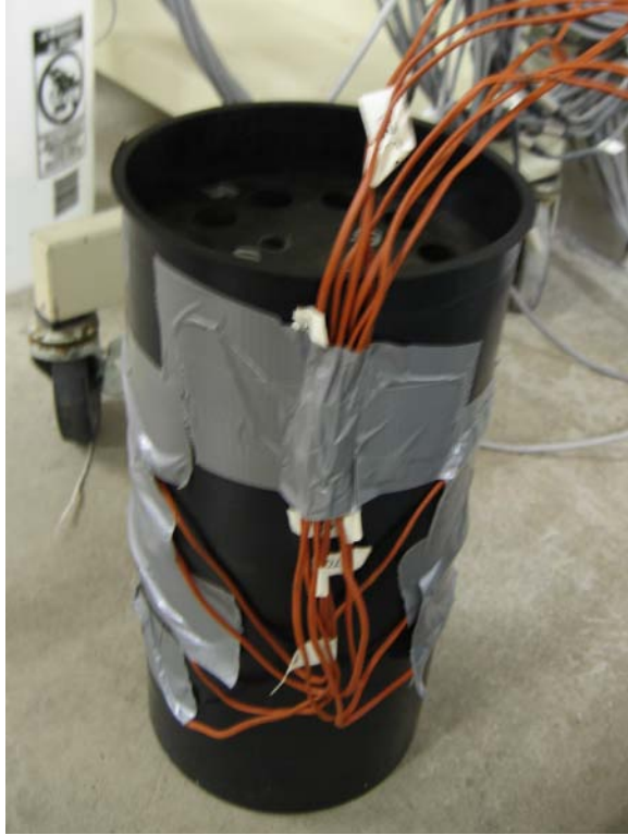
Figure 3.2: Sample instrumented with thermocouples.
