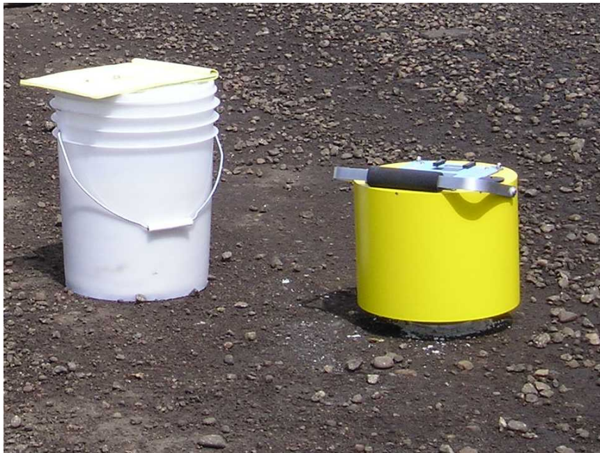
FIGURE 2.4 Soil stiffness gauge.
