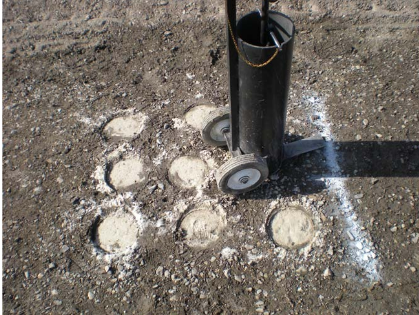
FIGURE 3.4 Testing with CIST to assess operator effects.
