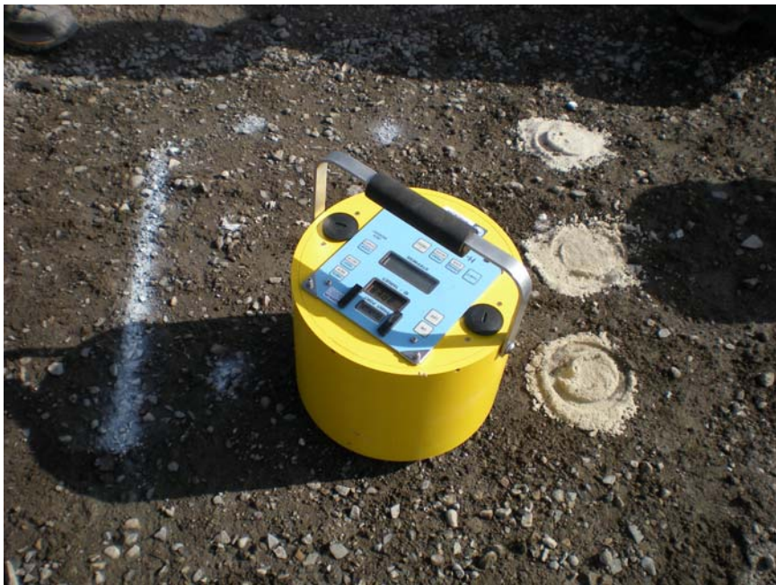
FIGURE 3.3 Testing with SSG to assess operator effects.
