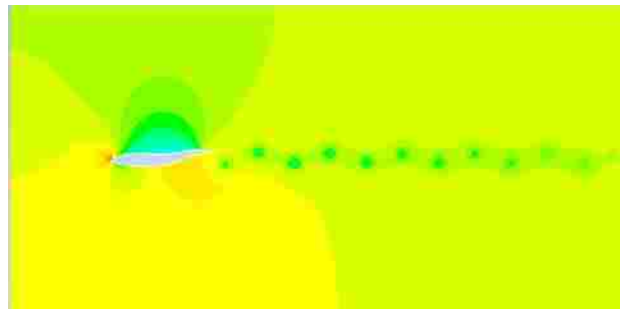
Figure 4-9: Pressure contour plots for the seventh tail beat of the LES simulation.
