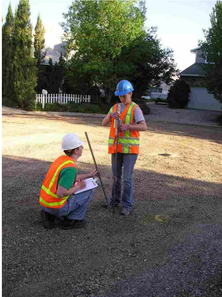
FIGURE 3.11 DCP testing just after reclamation.
