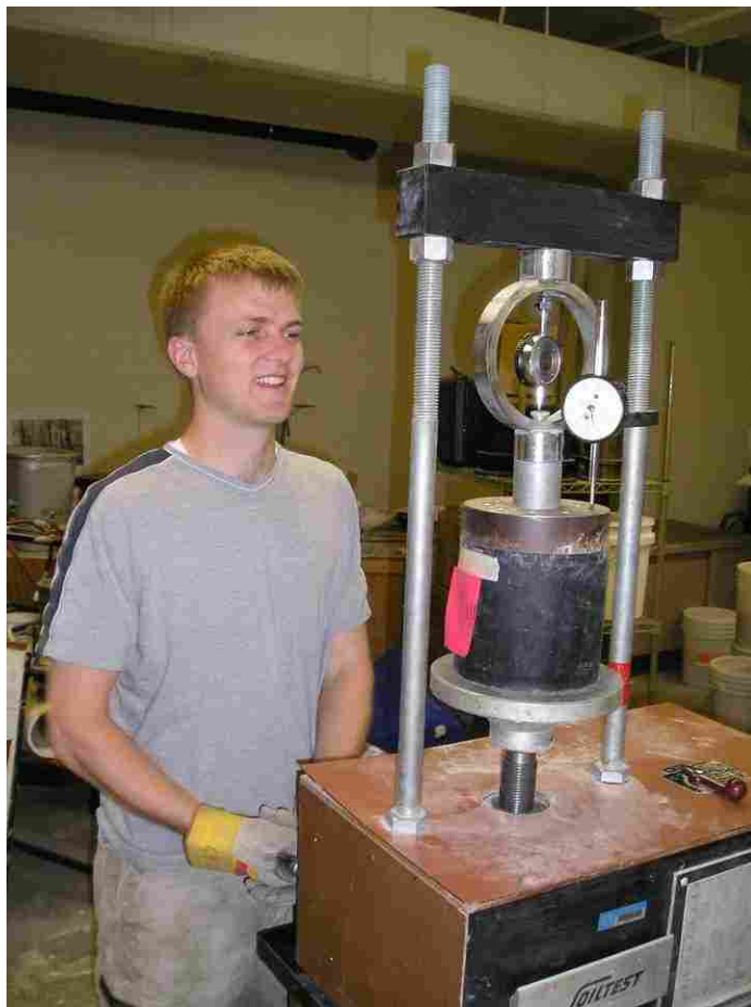
FIGURE 3.14 Compression machine used in CBR test.
