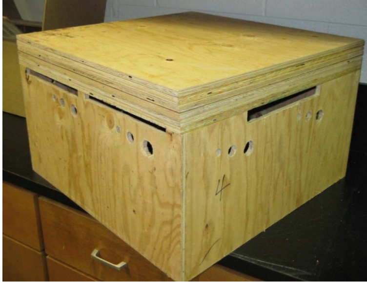
Figure 3-2: Completed cover meter testing apparatus.
