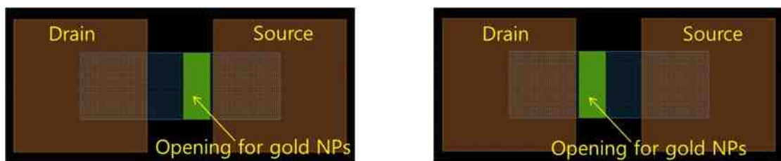
Figure 3.3 Mask design for the plasmon FETs with different positions of gold NPs. One device has the fabricated gold NPs near the source contact (left) while the other one has the gold NPs near the drain contact (right).
