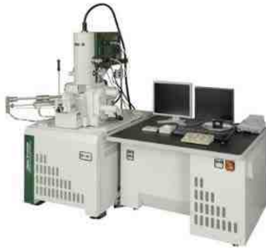
Figure 5.3 JSM-7100F Scanning Electron Microscope.
