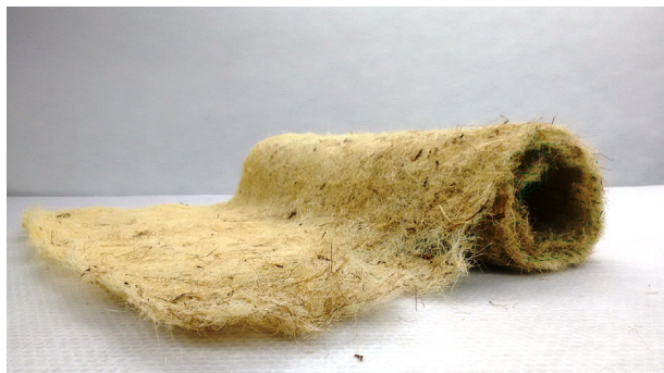
Fig. 1. Nonwoven industrial Fique Fiber mats.
