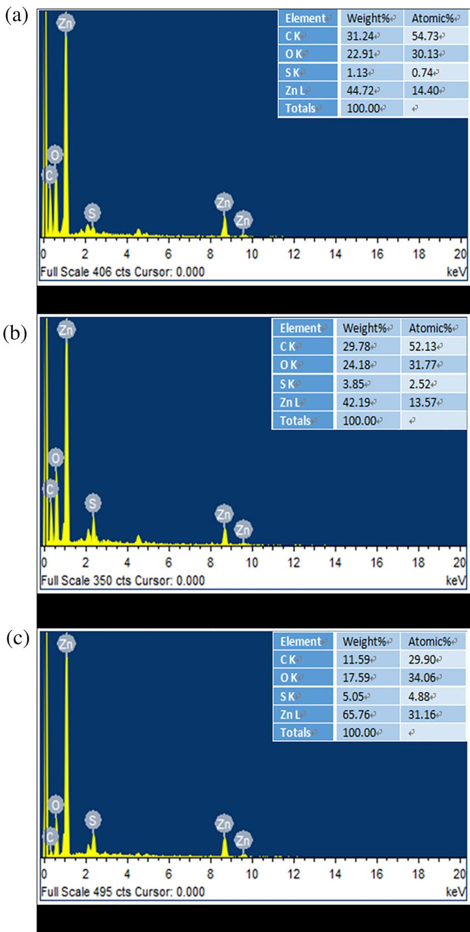
Fig. 6. EDS graphs of (a) ZnO nanostructures on a PET membrane and ZnO/ZnS core/shell nanostructures on a PET membrane under sulfurization times of (b) 10 and (c) 20 min.
