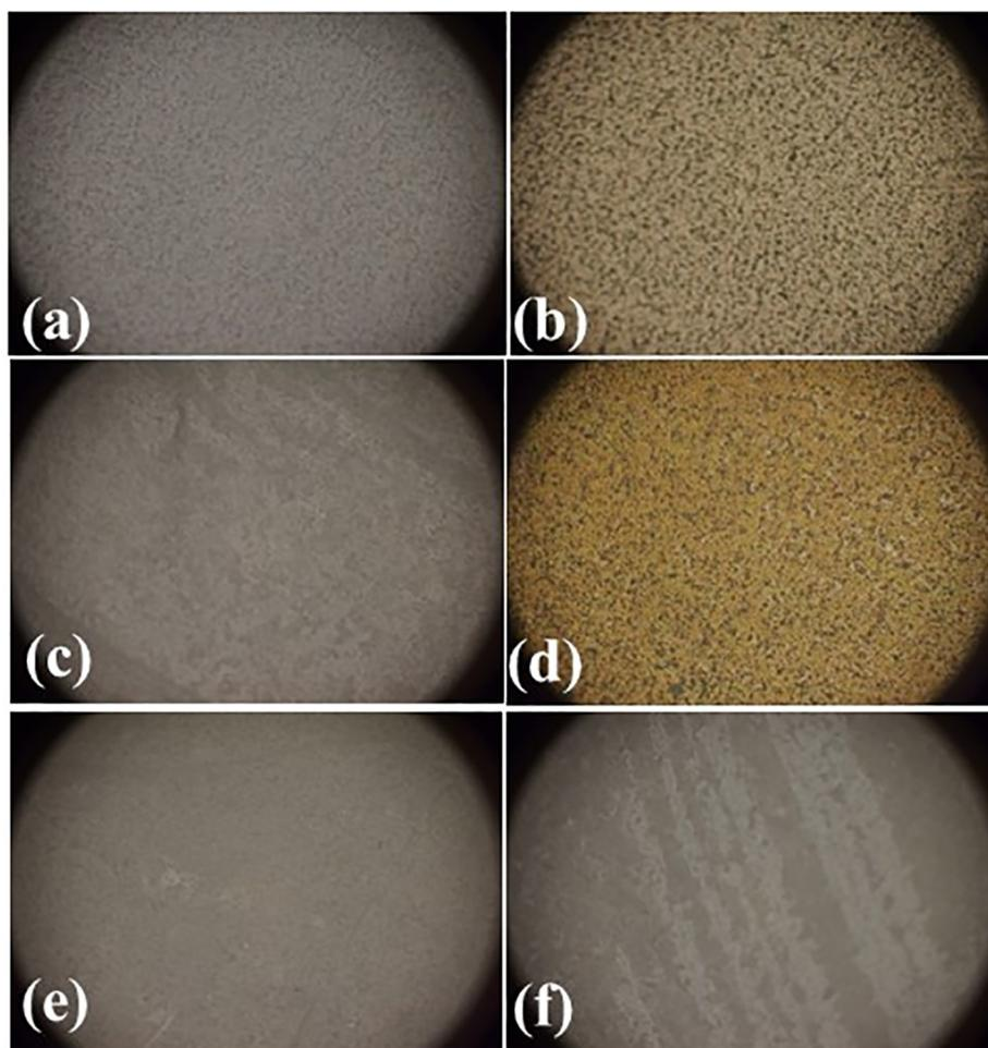
**Fig. 4.** Optical microscopic images of (a) a white PET membrane, (b) a PET membrane with a Au layer, (c) ZnO nanostructures on a PET membrane, (d) ZnO nanostructures on a Au/PET membrane, ZnO/ZnS core-shell structures on a PET membrane with a sulfurization period of (e) 10 and (f) 20 min.
