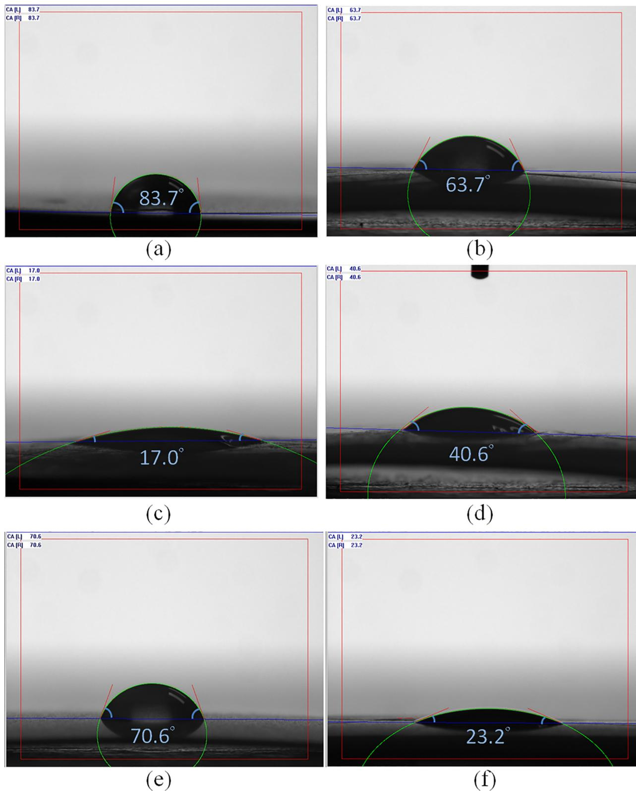
**Fig. 8.** Surface contact angle measurements of (a) a PET membrane, (b) ZnO nanostructures on a PET membrane, ZnO/ZnS core-shell structures on a PET membrane under sulfurization periods of (c) 10 and (d) 20 min, (e) a Au/PET membrane, (f) ZnO nanostructures on a Au/PET membrane.
