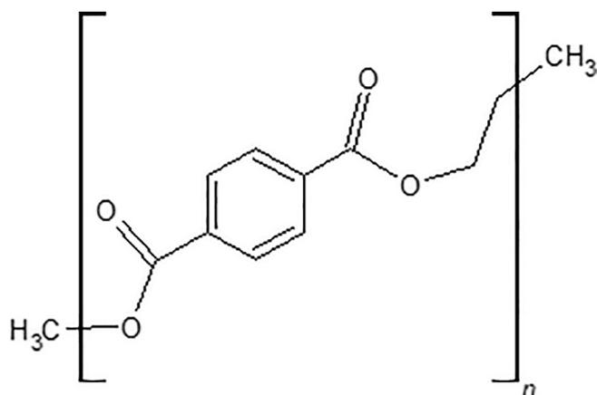
Fig. 1. Chemical structure drawing of PET.
