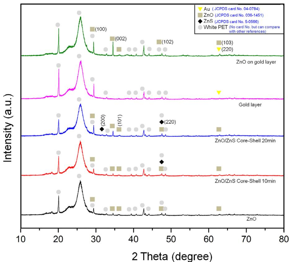
Fig. 5. From top to bottom: XRD patterns of ZnO nanostructures on a Au/PET membrane, a Au/PET membrane, ZnO/ZnS core-shell structures on a PET membrane under sulfuration periods of 10 and 20 min, ZnO nanostructures on a PET membrane.
