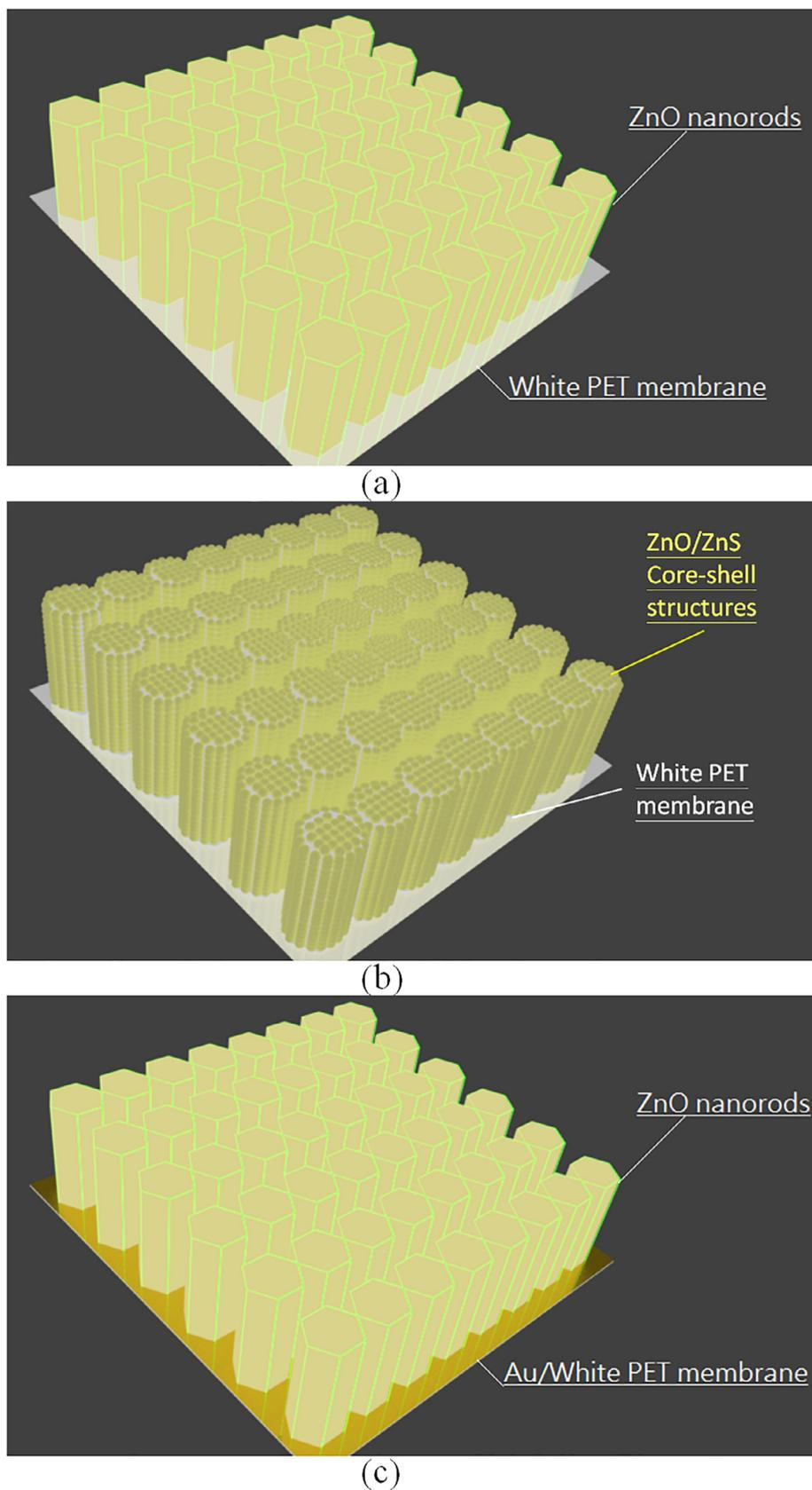
Fig. 3. Schematic pictures of (a) ZnO nanostructures on a white PET membrane, (b) ZnO/ZnS core-shell structures on a white PET membrane, (c) ZnO nanostructures on an Au/white PET membrane.
