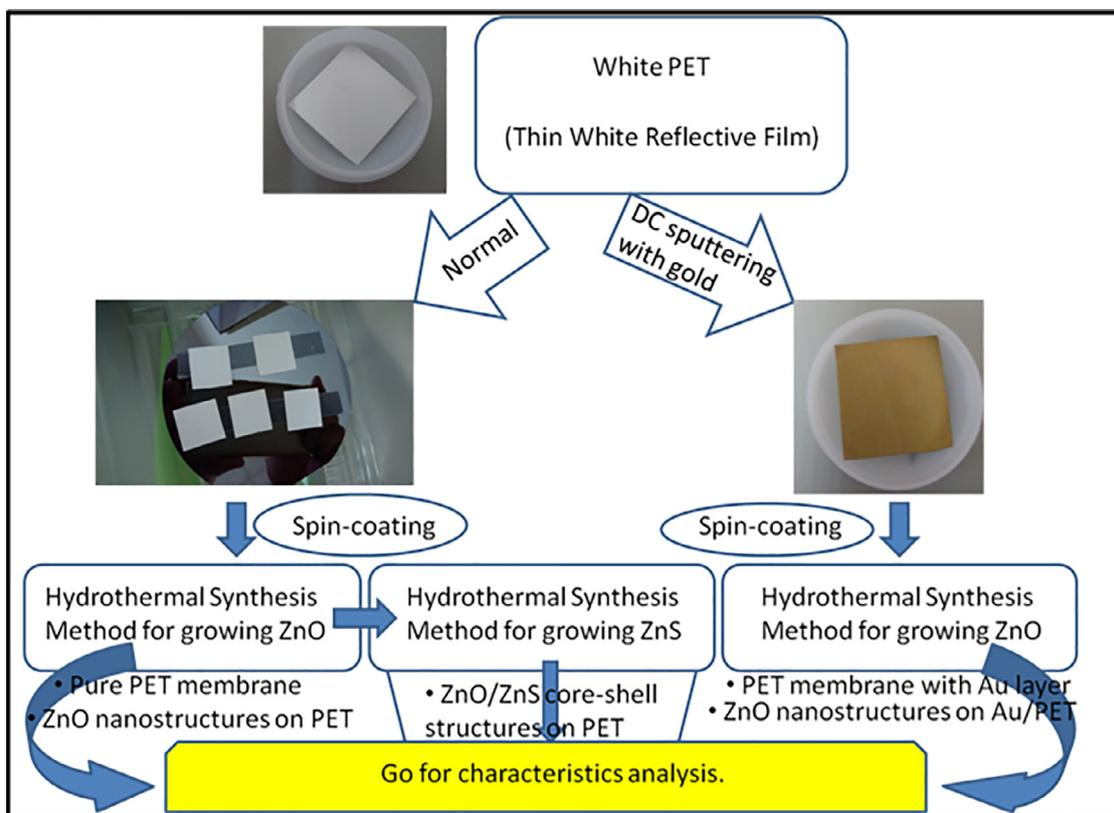
Fig. 2. Fabricating procedures of multi-layer reflective PET membranes.
