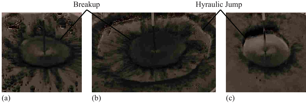
Figure 2.8: Sequence of images from CCD of jet impingement on a SH surface. Displayed are the three regimes of flow. Before the transition (a) only breakup can be seen and after (c) only a classic hydraulic jump occurs. The transitional regime (b) displays both breakup and a hydraulic jump.
