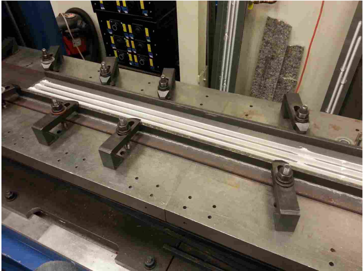
Figure D-4: Picture of setup for a 4' plate. Up to 3 welds were run next to each other on the same plate after the plate had cooled sufficiently.
