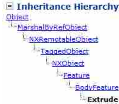
Figure 3.5: Inheritance structure for an extrude feature in Siemens NX 8.0 API
