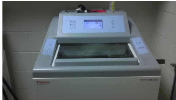
Figure 7-2: The cryostat was used to slice 8 \mu\text{m} thick transverse sections of the intervertebral disc stained with live/dead cell-staining medium.
