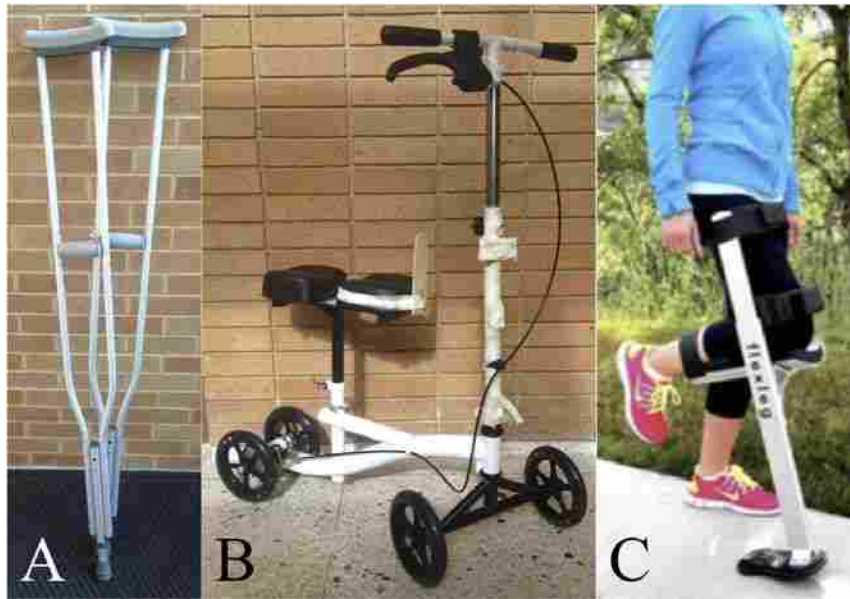
Figure 2-2: Crutches (A), knee scooter (B), and a temporary-injury prosthesis or TI prosthesis (C) used in the study.
