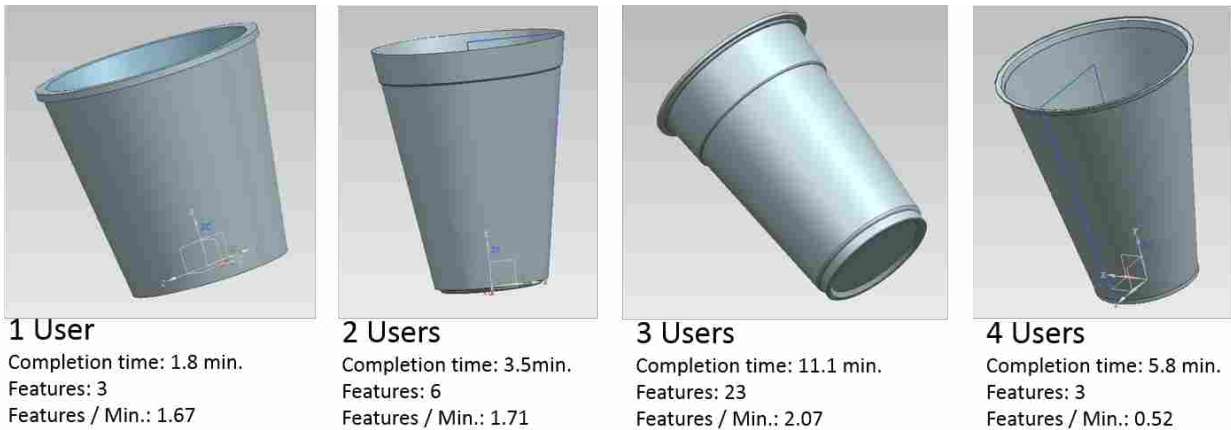
Figure 4.9: The level of detail included in the model of the cup generally increased with the number of users.
