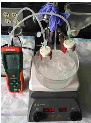
Figure D-1: Experimental apparatus used to monitor the increase in pressure due to O 2 generation during H 2 O 2 decomposition. Water maintained at a constant temperature holds test and control flasks on a hotplate while a differential pressure monitor measures transient pressure data.
