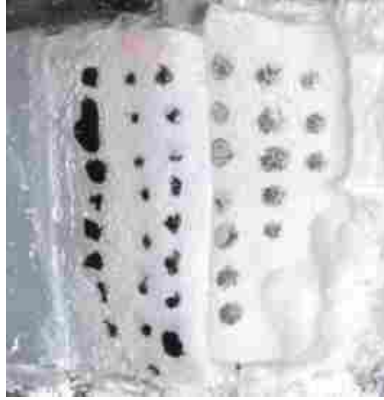
Figure 3.1: Grid of dots painted on the model to reduce error due to the correspondence problem.
