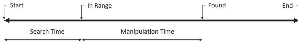
Figure 4.3: Events throughout a hotspot's active duration along a timeline. These include: start, end, in-range and found event times. Search and manipulation times are also visualized.
