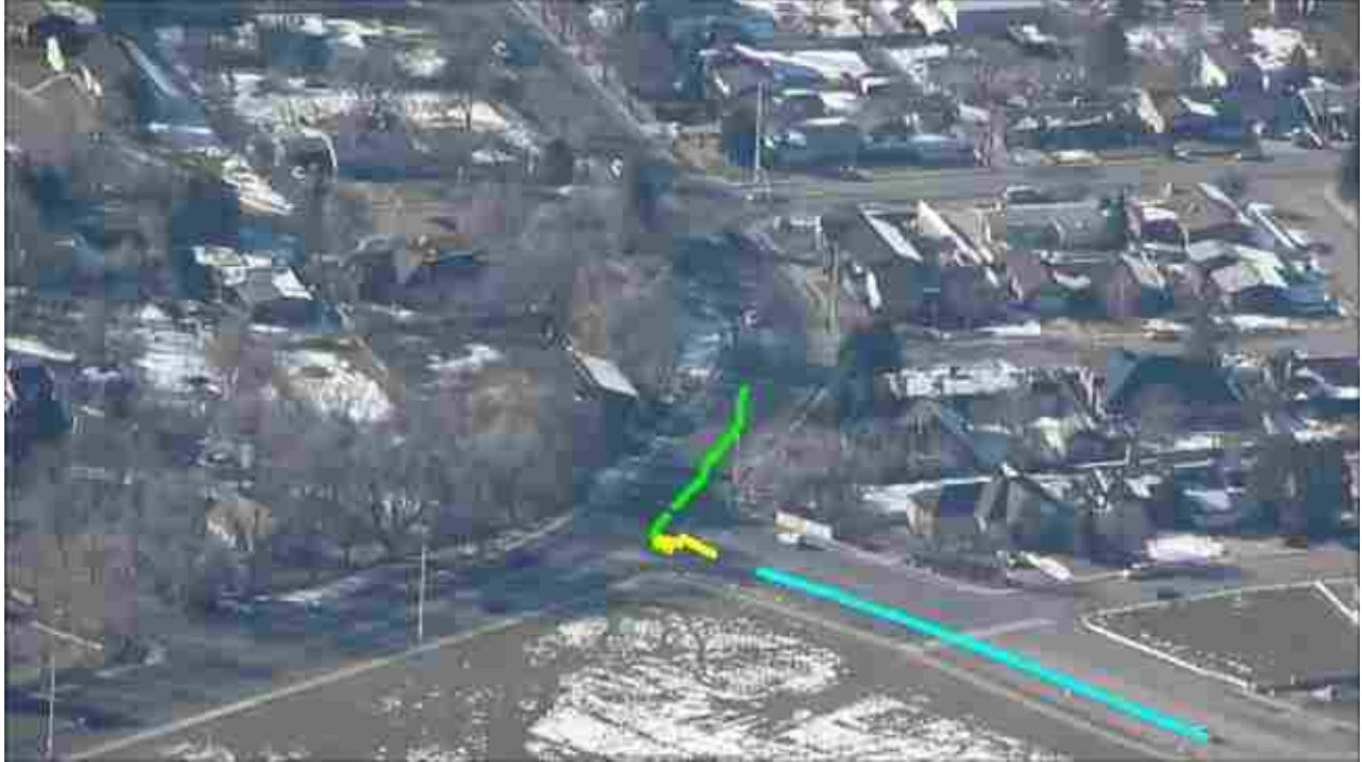
Figure 6.2: The R-RANSAC tracks associated with a car negotiating a left hand turn. This version of R-RANSAC uses the nearly constant velocity motion model and requires two new track initializations to complete the turn.
