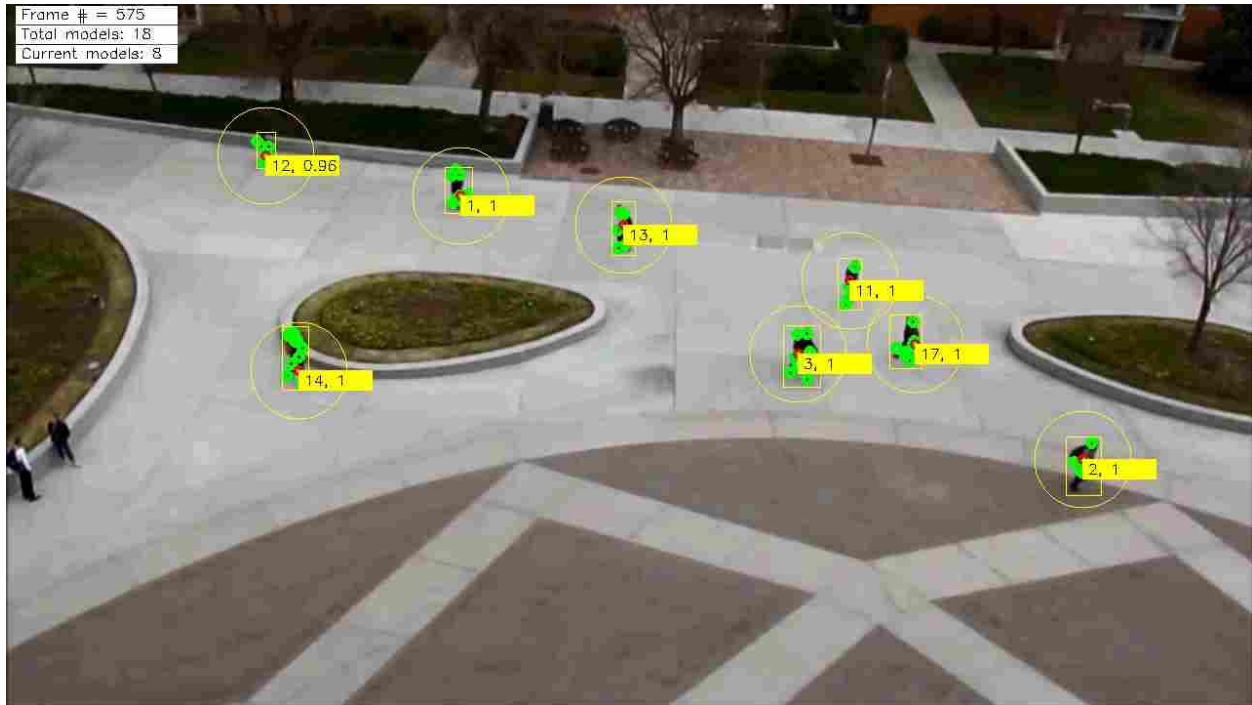
Figure 9.3: The video frame corresponding to Figure 9.2. Shown are the R-RANSAC tracks, their inlier regions, and the clustered measurements (in green).
