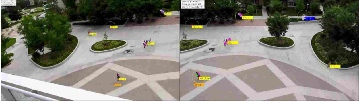
Figure 3.5: R-RANSAC can be used as a centralized tracker if measurements from multiple cameras are transformed into a common coordinate system. In this case, the measurements originating from the left panel are transformed into the coordinate system of the right panel. The homography is pre-calculated using manually selected feature pairs.
