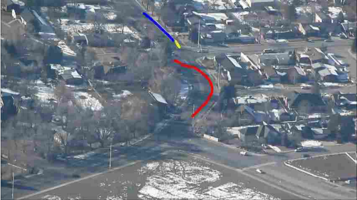
Figure 5.1: Three tracks produced by R-RANSAC with the nearly constant jerk model and nearest neighbor data association. The target of interest is briefly lost during the occluded intersection and then reacquired shortly thereafter.
