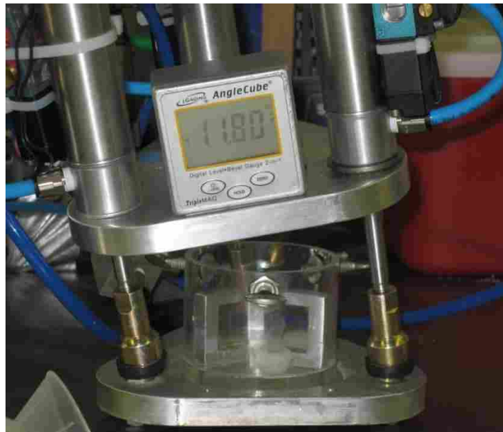
Figure 3-3: Magnetic bevel box used to measure angle displacement of bioreactor.
