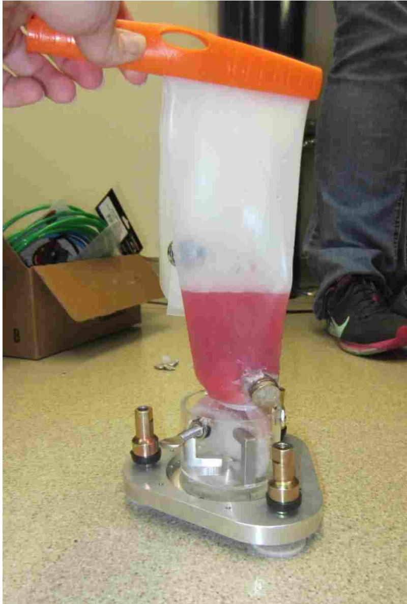
Figure 4-12: CamelBak bladder clip used to seal the silicone bag.
