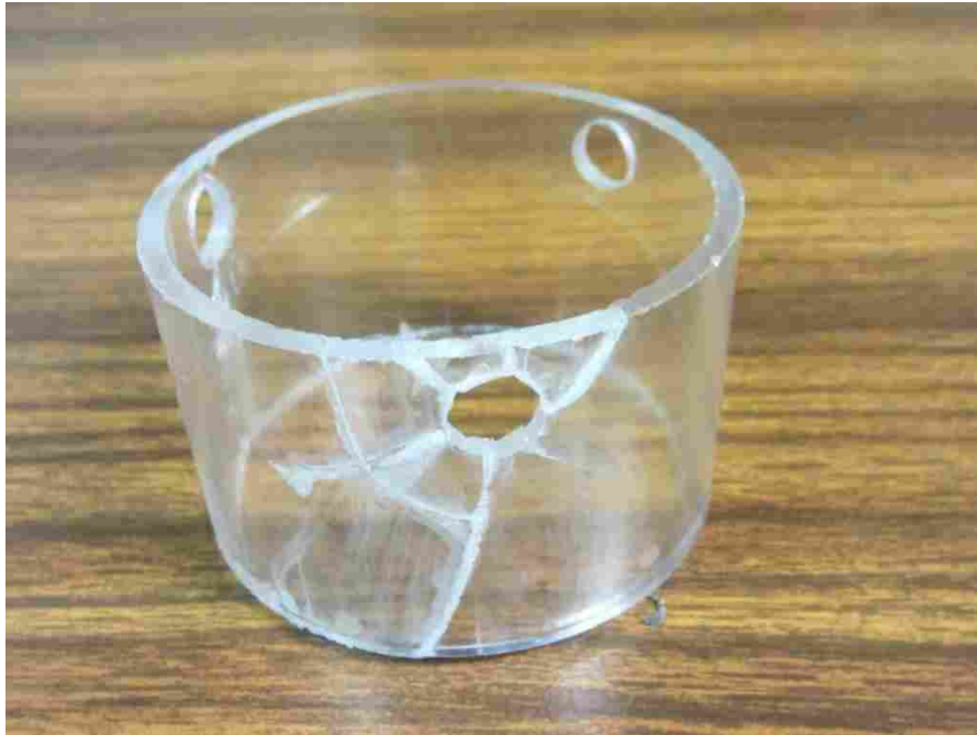
Figure 4-15: Shattered acrylic from the Gore valve.
