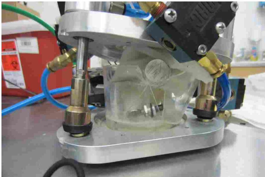
Figure 4-14: Gore valve causing the acrylic beaker to break.
