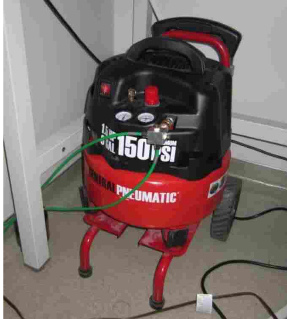
Figure 4-24: Air compressor used to supply air to the system.
