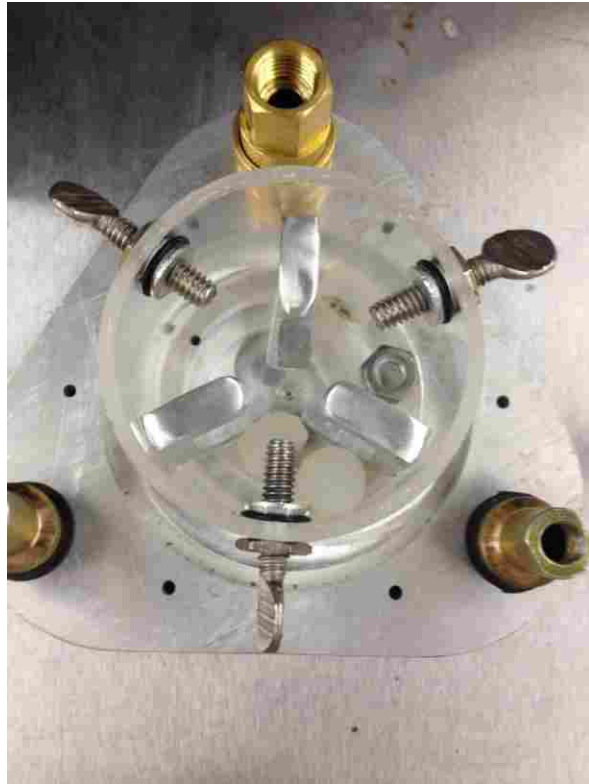
Figure 4-13: Thumb screw setup for securing the FSU.
