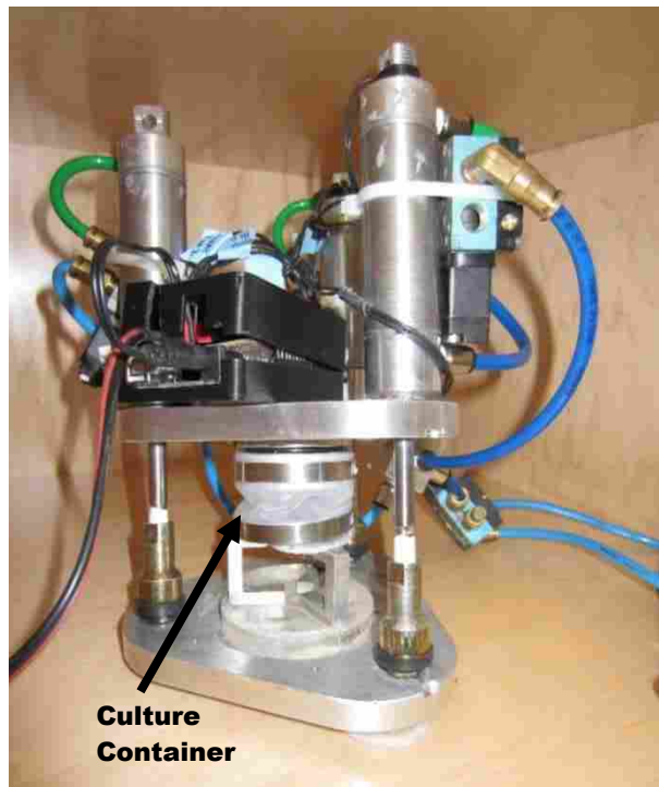
Figure 3-2: Complex loading dynamic bioreactor loading mechanism and culture container.
