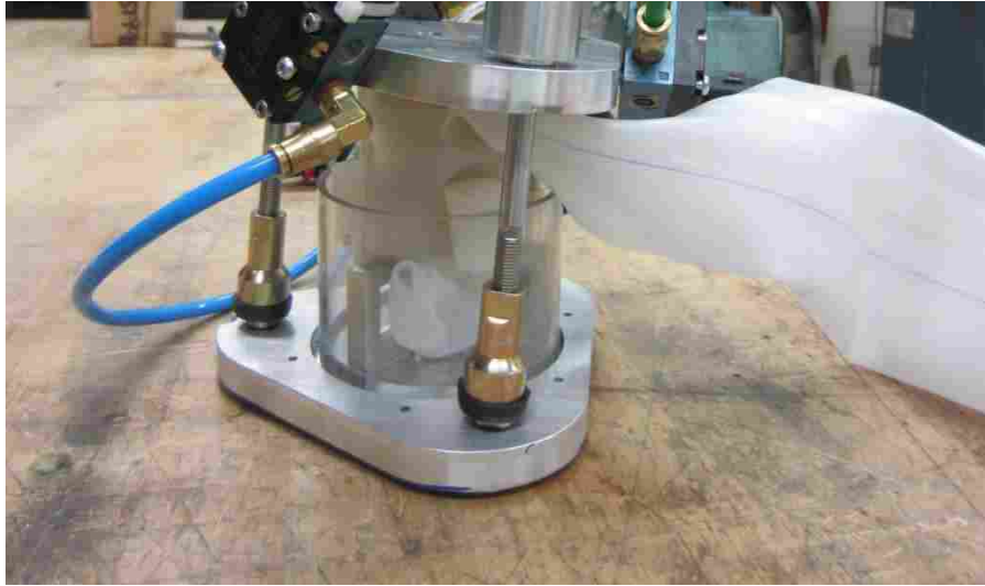
Figure 4-11: Semi-sealed container design with silicone stoppers.
