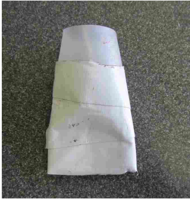
Figure 4-17: The silicone tube reinforced with fiber-reinforced adhesive tape.
