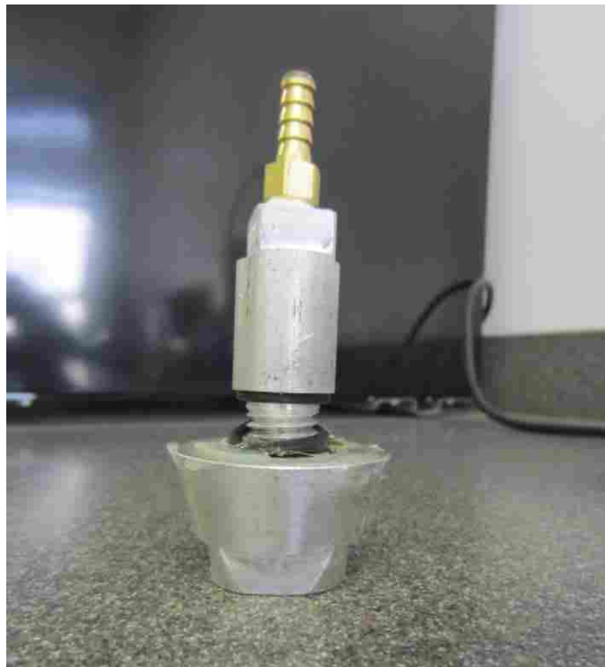
Figure 4-18: An aluminum version of the slanted seal with the vent protruding from the top.
