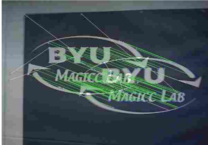
Figure 3.6: A superimposed image pair that was returned as a match by OpenFABMAP. A visual odometry algorithm computes the transform between the two images and returns it to be added in the pose graph. The transformation is visualized as the green lines overlaying the image.
