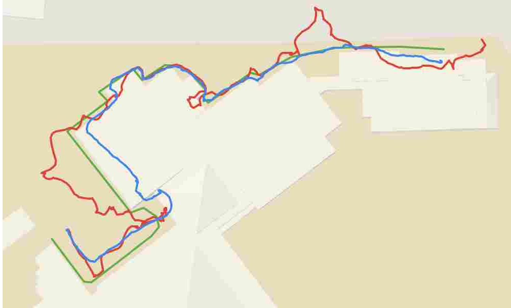
Figure 4.16: Comparison of refined maps using traditional and DCS least-squares optimization. The result of traditional least-squares (red) is clearly distorted as it uses all GPS measurements for optimization. The map refined using DCS (blue) rejects erroneous GPS measurements and results in a more consistent and globally aligned map. The true experimental path is displayed in green.
