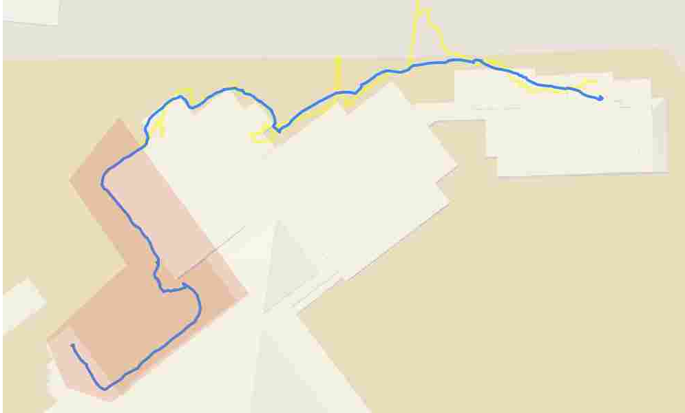
Figure 4.17: Demonstration of rejecting initial erroneous GPS measurements to compensate for initial bias. The red-shaded region corresponds to the area that GPS measurements are rejected.
