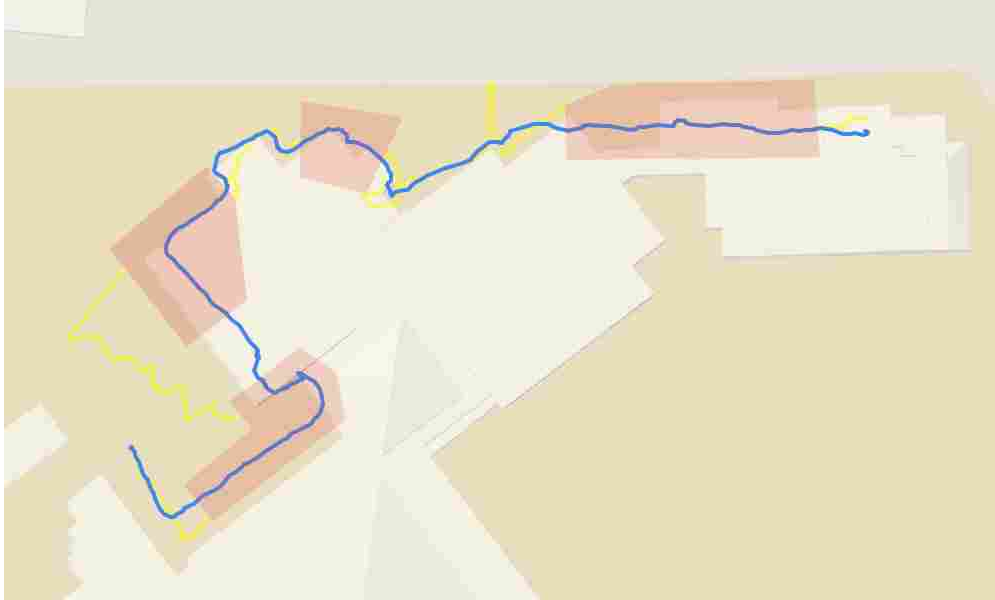
Figure 4.18: Maintaining globally consistent and aligned maps in the presence of non-uniformly intermittent GPS measurements is demonstrated by artificially creating GPS-denied regions. The red-shaded polygons indicate the GPS-denied areas. The optimized path is displayed in blue.
