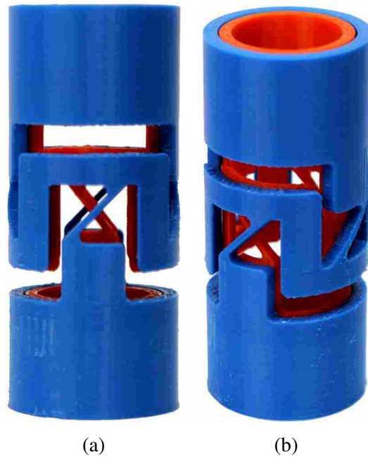
Figure 2.23: 2 DoF CCAFP prototype with intersecting axes of rotation. Blue and orange PLA was used to differentiate between the inner and outer tubes, respectively.
