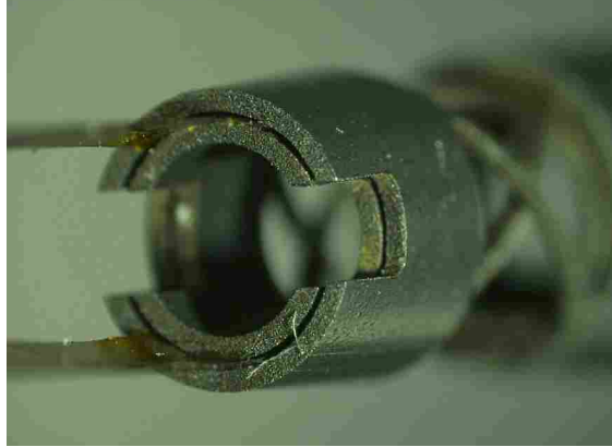
Figure 2.16: 3 mm NiTi CCAFP with Kapton shims before bonding the inner and outer cylinders.
