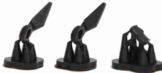
Figure 3.13: 6 mm L-Arm SLA parts shown in the as-manufactured state, including support material.
