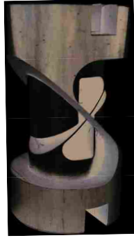
Figure 2.9: 4130 steel CCAFP with cam-surface integrated in the inner cylinder.
