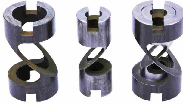
Figure 2.5: CCAFP made of 4130 steel. The outer cylinder OD is 1.125 in (28.6 mm). The height of each cylinder is approximately 2 in (51 mm).
