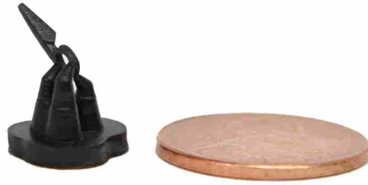
Figure 3.12: 3 mm L-Arm SLA jaw (with support material) shown next to a US Penny for scale.
