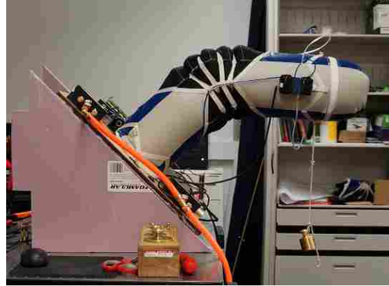
Figure 3.7: Experimental set-up for stiffness validation at approximately 45°
