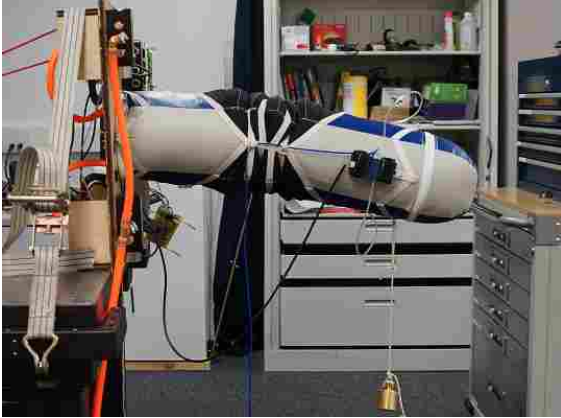
Figure 3.6: Experimental set-up for stiffness validation at approximately 0°
