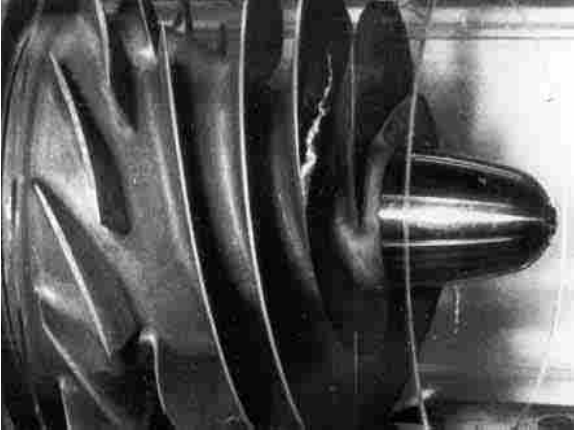
Figure 2.2: Tip vortex cavitation on Impeller. Image taken from Brennen [2]
