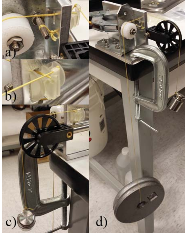
Figure 2.16: Test fixture used to test design variants A) cable holding joints in compression B) custom 3D printed joints with moment arm C) weight applying torsional load D) weight keeping joint in compression
