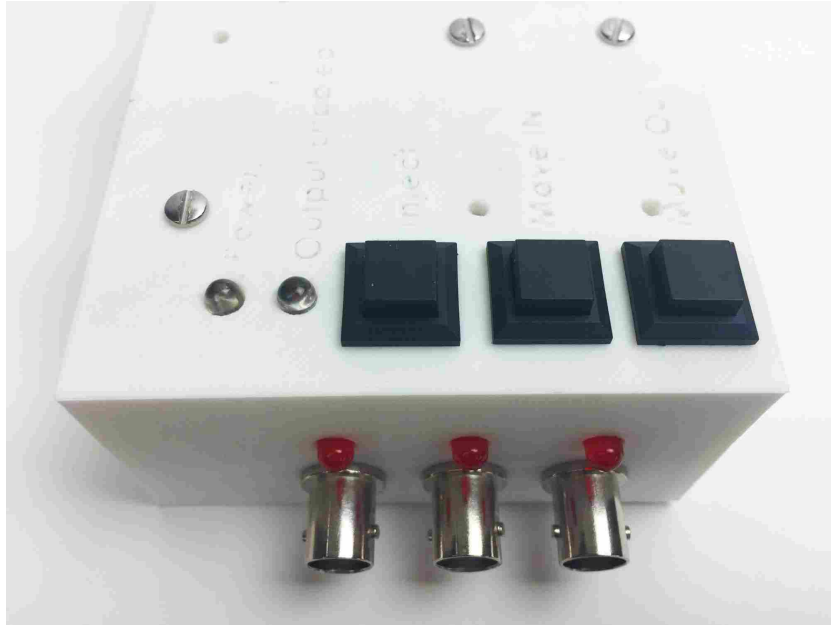
Figure 5.3: User interface on the automated injection control box.
