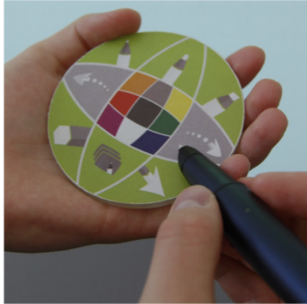
Figure 2.3: Close-up of the Pen and Tool Palette Used With the Interactive Whiteboards [1]
