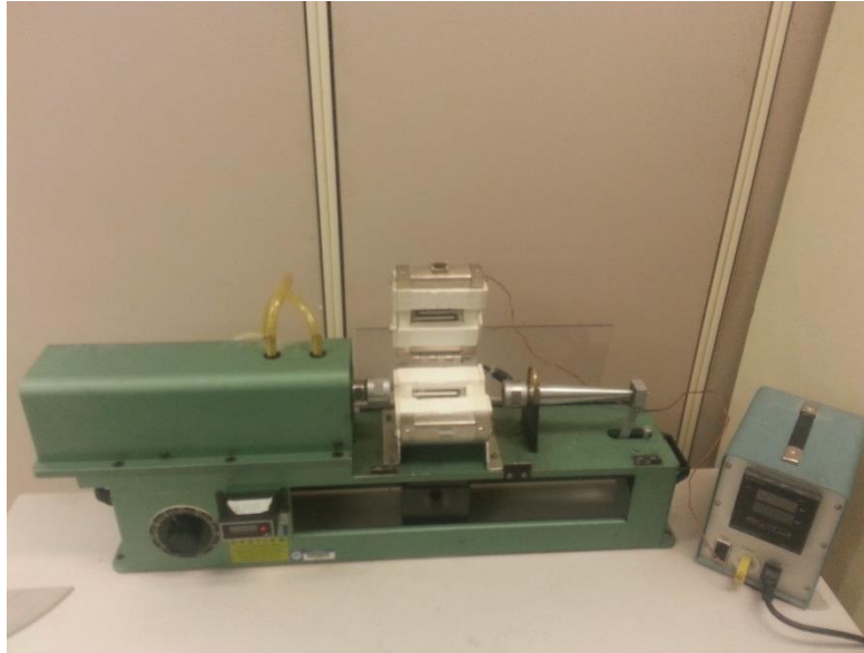
Figure 3-1: Rotating-bending fatigue machine with mounted furnace and adjacent temperature controller.
