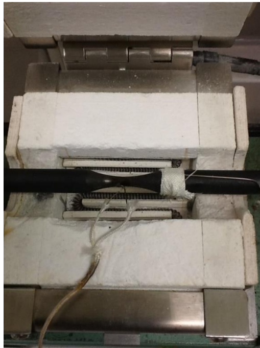
Figure 3-3: Thermocouple attached near minimum cross-section via welding.
