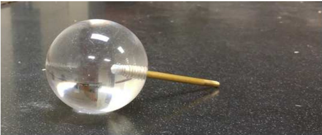
Figure 3.4: Sphere for determining Flow Regime in Wind Tunnel
