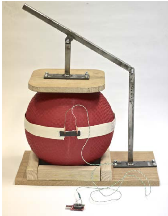
Figure 4.3 – Contraction simulator. A utility ball is depressed and released to simulate the circumferential change of the abdomen.
