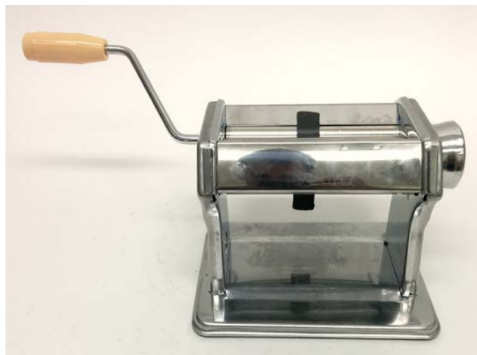
Figure 2.5 – Crank roller used for pre-conditioning gauges to reduce the effects of permanent deformation.
