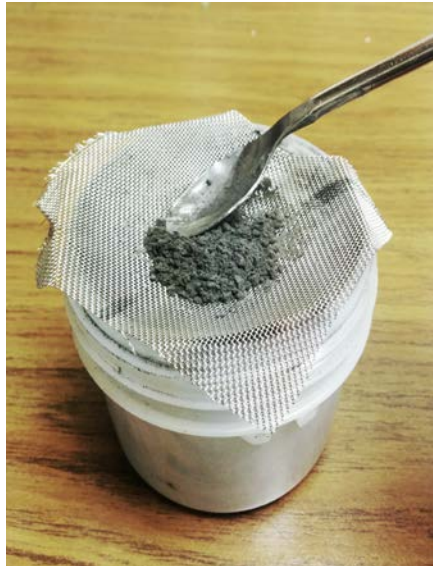
Figure 2.2 – NiNs being forced through a wire mesh. This process is known as “screening”
