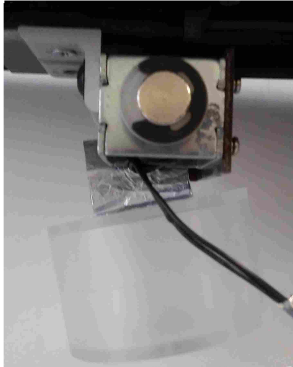
Figure 2.4: Solenoid drop mechanism holding the buoyant cylindrical puck used in this study. The angle of the puck depends upon the attachment point on the aluminum foil tab.
