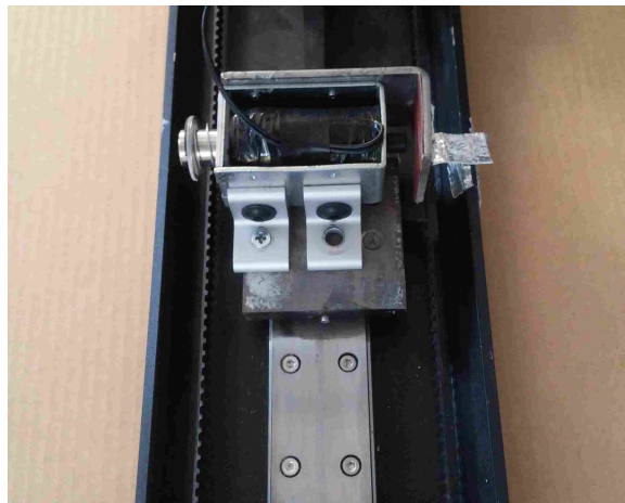
Figure 2.5: Side view of the solenoid drop mechanism attached to a belt driven actuator. The belt was driven by a stepper motor which was controlled using LabVIEW. The aluminum foil tab extending off of the end of the drop mechanism is what the photoelectric sensor detects at the end of the track.
