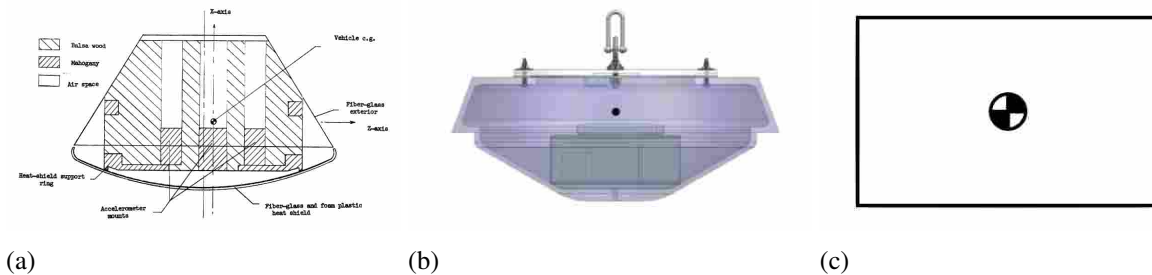
Figure 3.25: A side by side comparison of the three different shapes that have been tested for inversion characteristics. A cross section of the 1/4 scale Apollo command module [12] (a), the 1/8 scale TiME capsule [26] (b), and the cylindrical puck (c) are shown. The center of gravity is different in each case.
