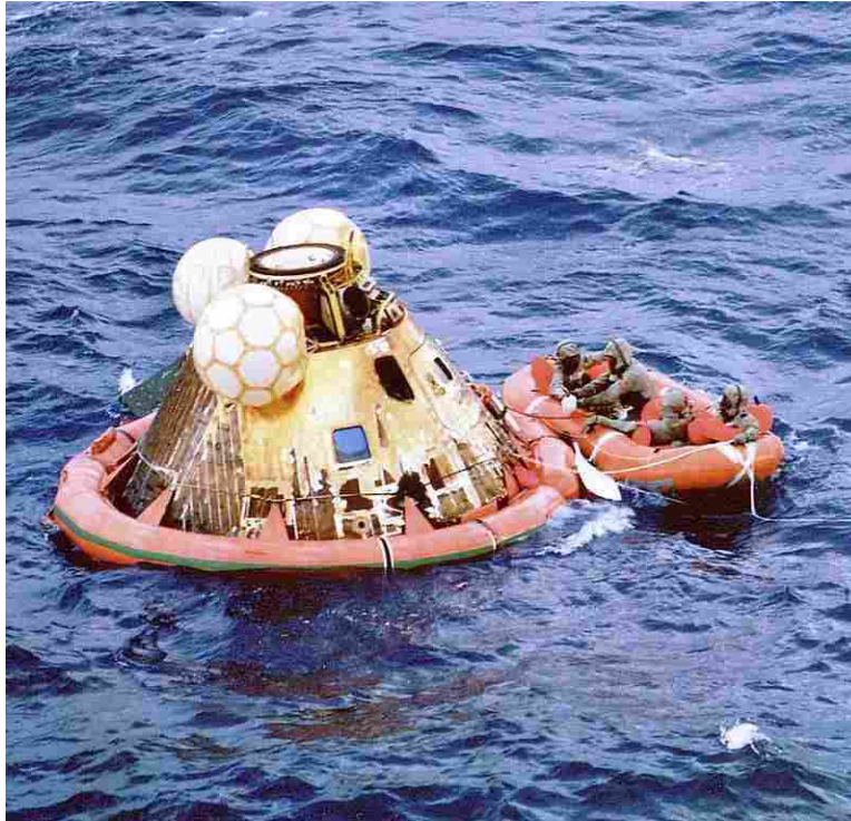
Figure 1.3: Recovery of the Apollo 11 spacecraft. During this mission the spacecraft inverted upon splashdown. The airbags were deployed to flip the capsule back to its upright orientation. (NASA)
