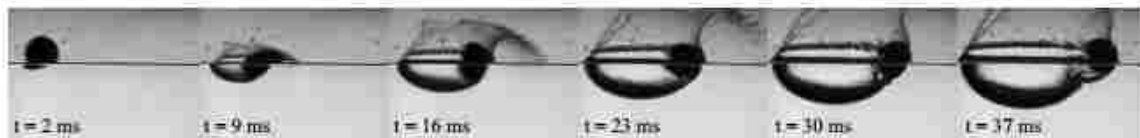
Figure 1.10: Image sequence for a deformable sphere skipping on water. A hydrodynamic lift force causes the sphere to leave the cavity before the cavity collapses [29].
