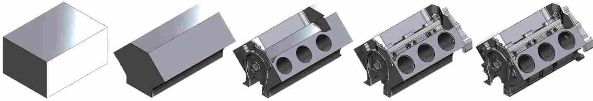
Figure 2.3: Typical serial progression of operations for an engine block
