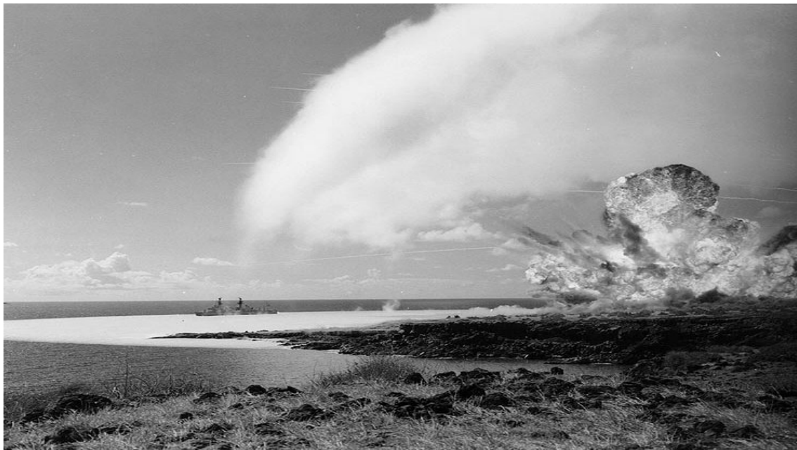
Figure 4.1: The first of a series of three detonations during Operation Sailor Hat in 1965. 500 tons of TNT were detonated to simulate the effects of a nuclear explosion. Public domain image.
