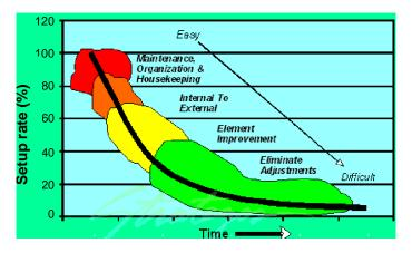
Figure 1. Phases of Set up Reduction.
