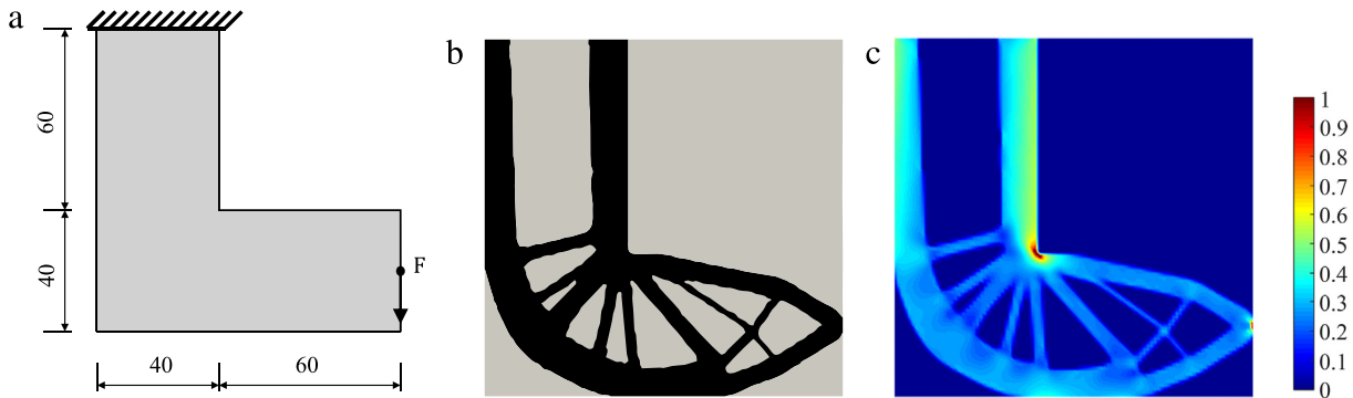
Fig. 7. L-bracket example explored by Allaire and Jouve [16]: (a) design domain with midpoint load; (b) our solution using p -norm sensitivities with p = 2 and (c) the correspondent von Mises stress field.
