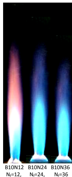
Figure 9. Effect of the number of fuel ports on the Flame configuration at air Reynolds Number 7831 ( \Phi_p=1.2 ) for burner B10.
