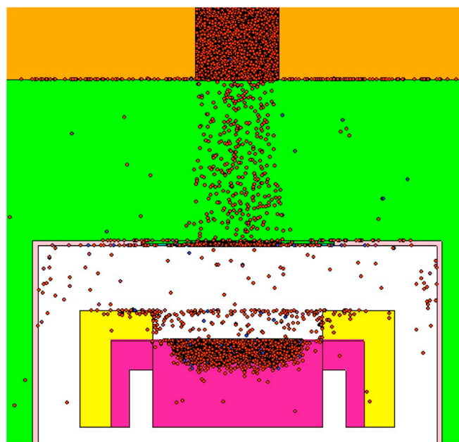
Fig. 3. Tracking of the interactions of photons with energy of 11.87 keV inside the model of Si(Li) detector for measurement configuration with collimator.
