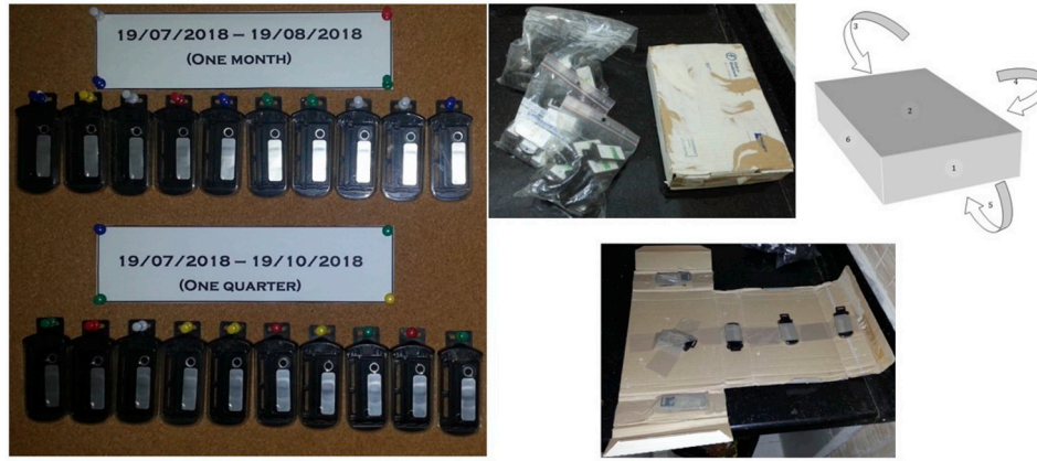
Fig. 1. Sets of dosemeters used to measure monthly and quarterly natural radiation background doses in the DGRSN's IMS laboratory (left). Packages and box sent to the organizing SSDL (right). In particular, the 6 transport and radiation background dosemeters fixed on each face of the box are shown.
