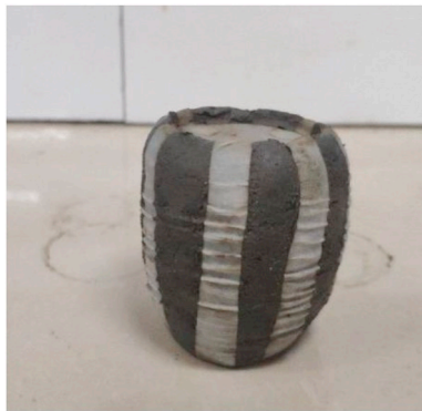
Fig. 8. Soil sample compression failure.
