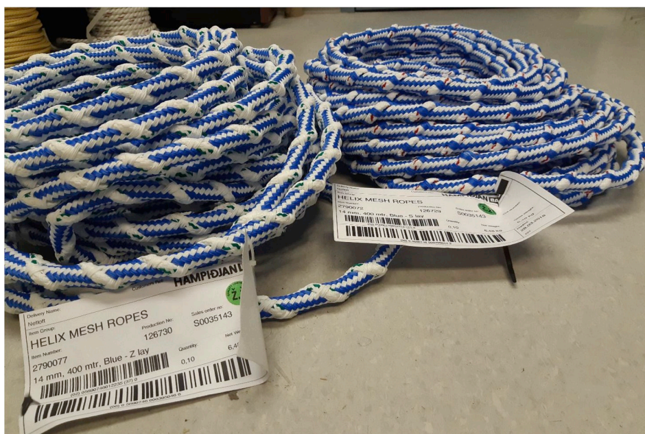
Fig. 1. Sample of 14 mm helix ropes of S-lay in left side and Z-lay on the right side.
