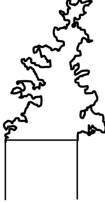
Figure 2.3 Instantaneous edge of a highly contorted flame front [27].
