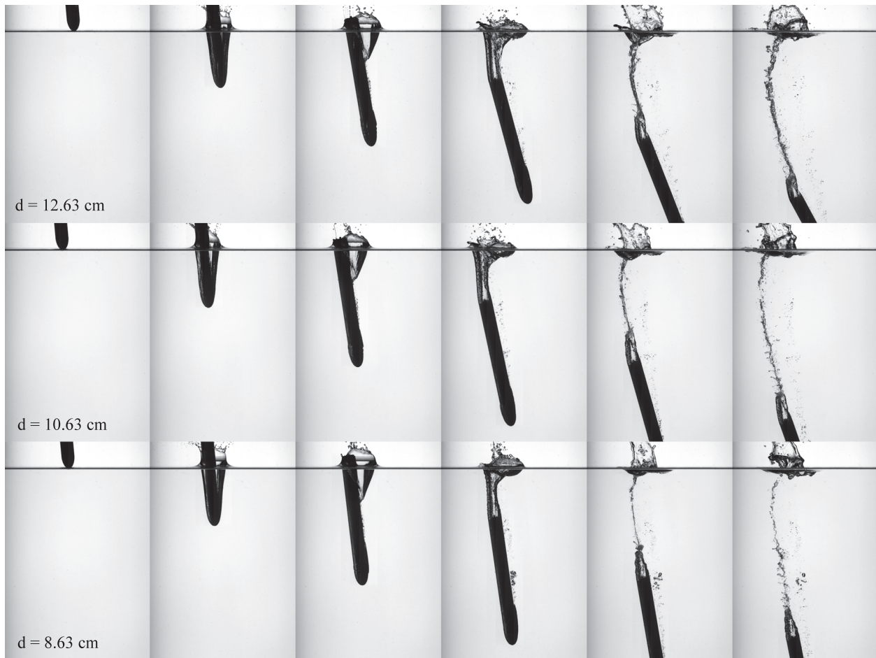
Figure 3.10: Image sequences of a modified hydrophobic Delrin ogive dropped from 50 cm with the center of mass located at 12.63 cm, 10.63 cm, and 8.63 cm from the nose of the projectile. The time between each image is 32.0 ms and the impact velocity was 3.1 m/s.
