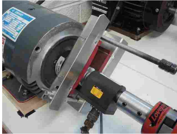
Figure 3.9: Mechanical Braking Device used to Simulate Loading
