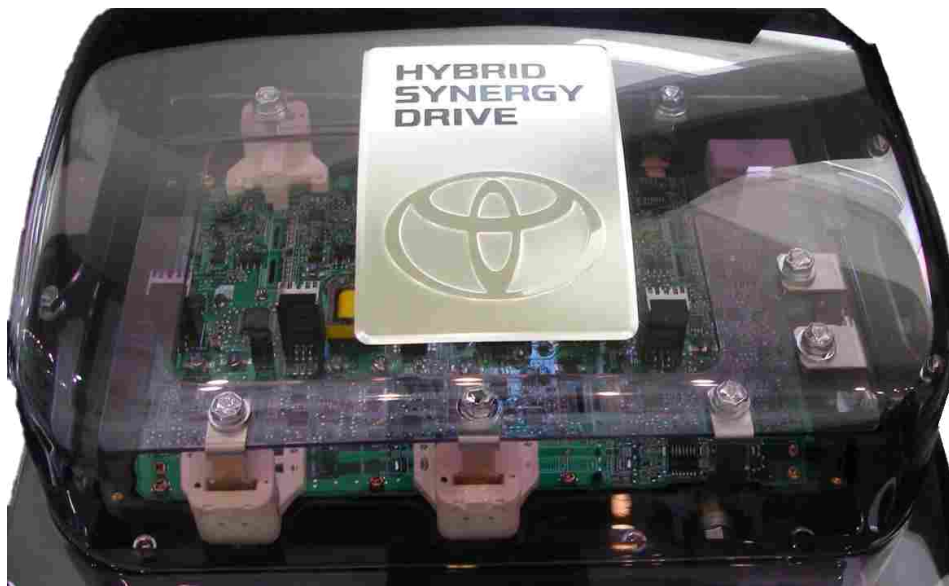
Figure 1.2: Electronic Controller for the Toyota Prius
