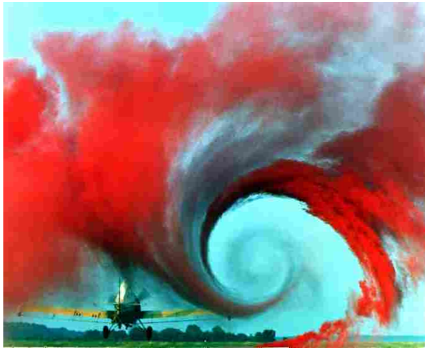
Figure 2.2: Wingtip vortex visualized with smoke. Photo taken from [21].
