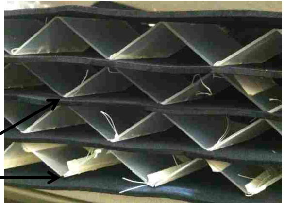
Figure 6 – Side view of crash pad design showing layering of Miura-ori and elastic membrane.
