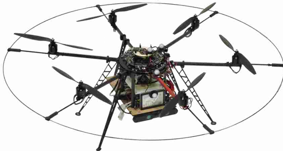
Figure 1.5: The Mikrokopter hexacopter prototype that we use in experiments discussed in this research. The only sensors we utilize are an altimeter, IMU, and front-facing RGB-D camera. All computation is completed onboard the vehicle and it communicates with a ground station computer using 802.11n Wi-Fi. The groundstation only provides goal locations to the platform.
