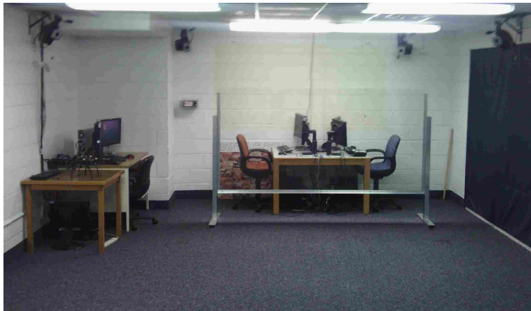
Figure 2.8: Here is the motion capture environment where all the testing was conducted for this research. We use a motion capture system from Motion Analysis. The system provides 6DoF pose information at 200 Hz with sub-degree and sub-millimeter accuracy.
