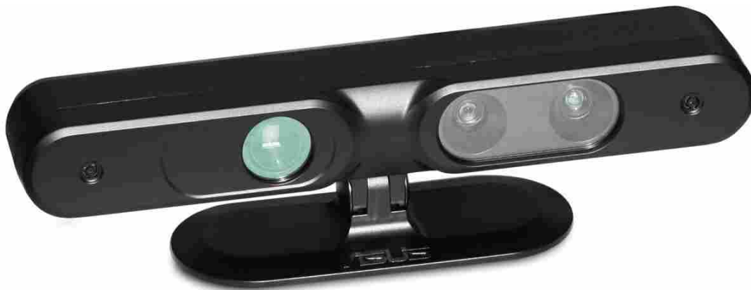
Figure 1.7: An RGB-D camera provided by ASUS. The infrared (IR) projector is on the left, the regular RGB camera in the middle, and the IR receiver is on the right. Dense stereo processing, which is completed on the device, is used on the projected IR points to find the depth in the scene.
