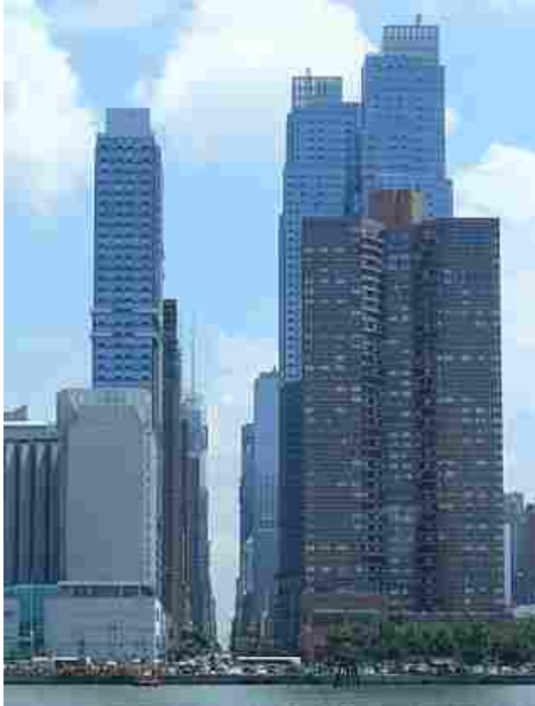
Figure 1.3: An example of an urban canyon. The tall buildings obstruct and create multi-path effects for GPS signals. Small UAS must be robust to degraded or intermittent GPS signals for flights in these areas. Photograph ©Ad Meskens, used with permission.
