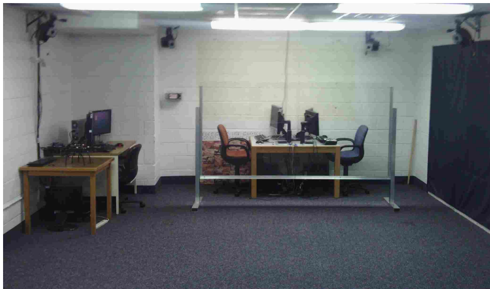
Figure 1.6: Pictured is the motion capture environment from Motion Analysis where most of the testing was conducted for this research. The system provides 6DoF pose information at 200 Hz with sub-degree and sub-millimeter accuracy.
