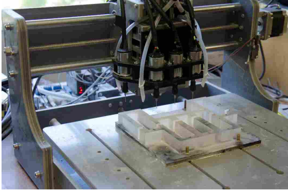
Figure 3.6: CNC mill with 5-bit array adaptation and milling fixture.
