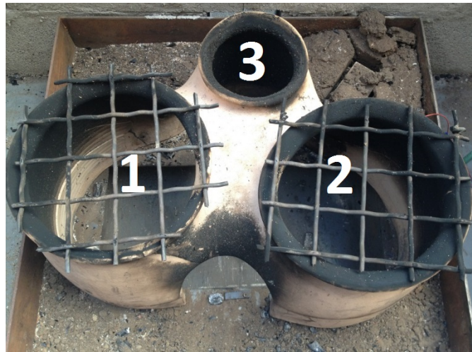
Figure 2-3: Top view of Peruvian cookstove.
