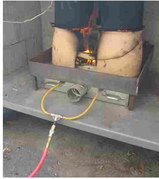
Figure 2-10: Biogas tank with regulator and flow meter. Biogas connected to burners.
