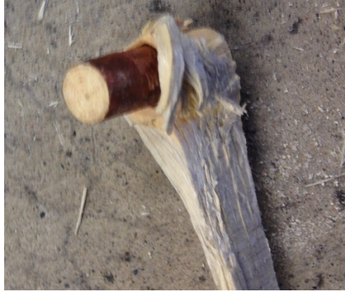
Figure 3-34: Knot randomly distributed in the test wood
