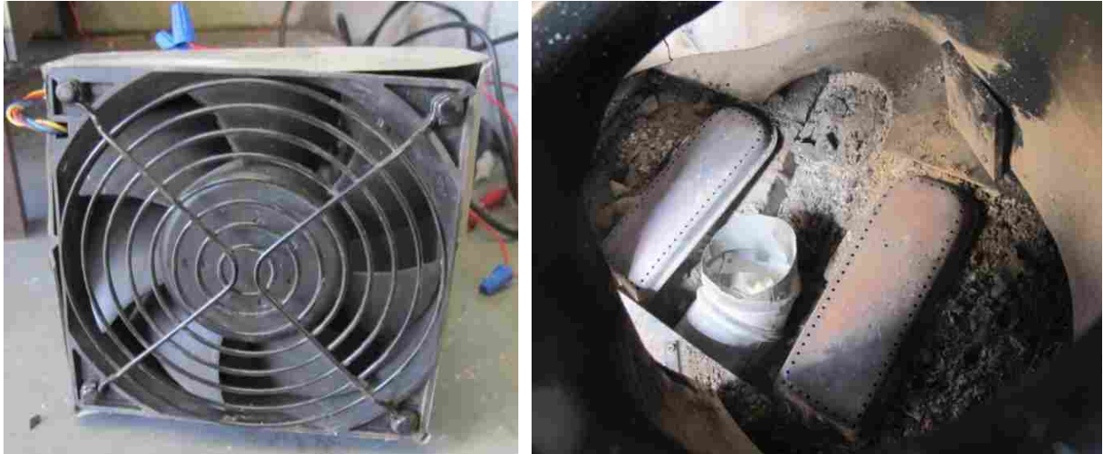
Figure 2-4: Fan to provide air. Two burners to deliver biogas and a duct to supply air.
