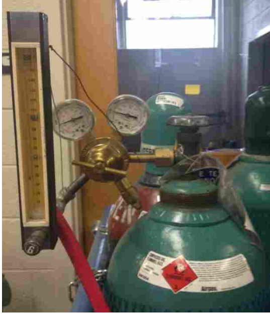
Figure 2-10: Biogas tank with regulator and flow meter. Biogas connected to burners.
