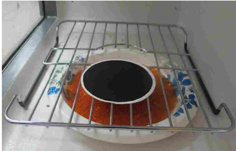
Figure 2-5: Filter paper being desiccated. Filter paper being weighed on microbalance.
