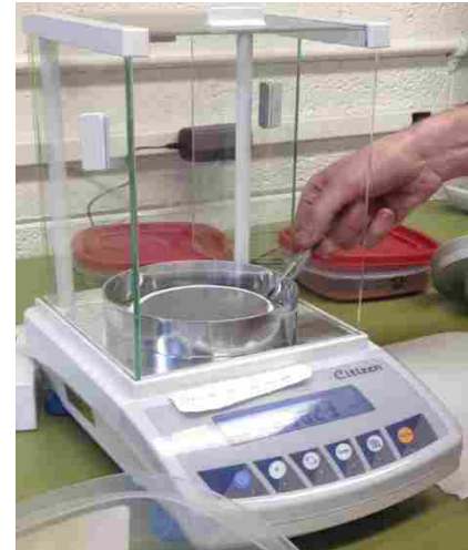
Figure 2-5: Filter paper being desiccated. Filter paper being weighed on microbalance.
