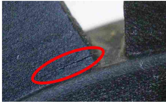
Figure 3.12: Crack in the manifold.
