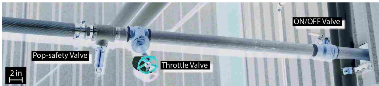
Figure 3.5: ON/OFF valve, throttle valve, and pop-safety valve. The pipe size in this figure is 2 inches.
