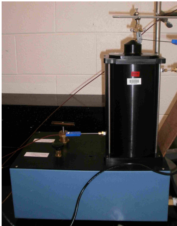
Figure B.1: TSI 1127 Air Velocity Calibrator.
