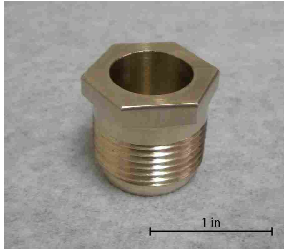
(b) Ball valve stem bearing.
