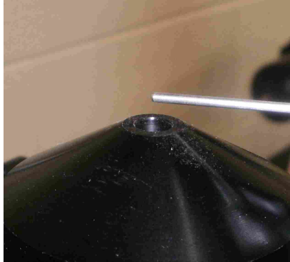
Figure B.4: Thermocouple position above nozzle.
